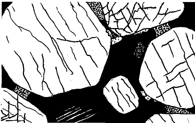
Figure 3 - Drawing based on a polished thin section showing the shapes and distribution of the meteorite constituents. Width: 2.5 cm. Black interstitial mass: kamacite (and taenite in lamellar intergrowth, seen at lower left). Large idiomorphic crystals are olivine. Other minerals shown: troilite (heavily stippled) schreibersite (lightly stippled), chromite (checkered). Kamacite - taenite intergrowth is a feature revealed in a SEM preparation and inserted herefor whole-
